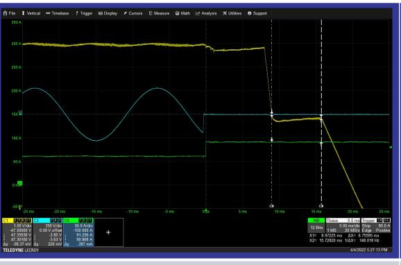
To meet minimum 6msec, the bulk energy depleted trigger was set from 66.6% down to 50% (30J). This remaining energy can sustain output at 48V for at least 6msec with 150% load.
