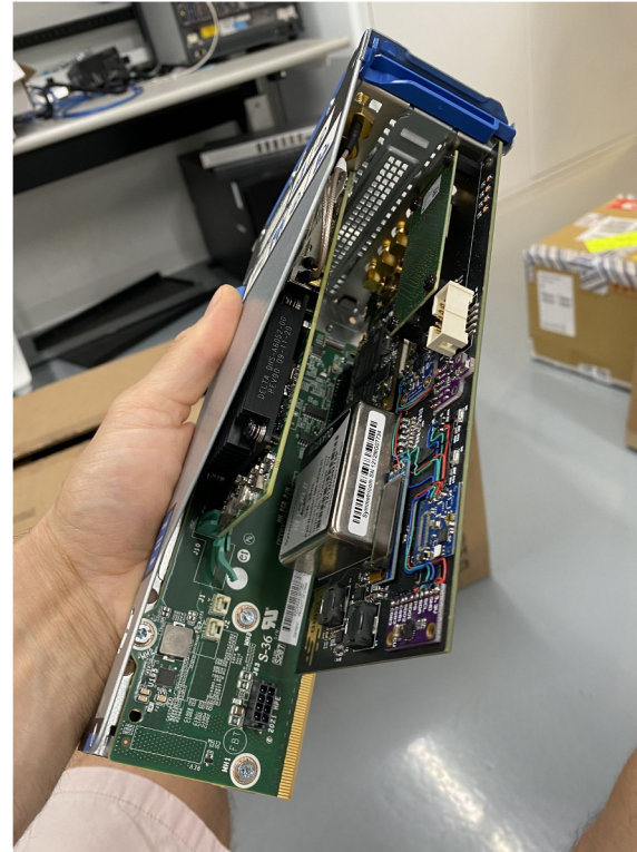
HPE Raiser designed for Time Appliance
