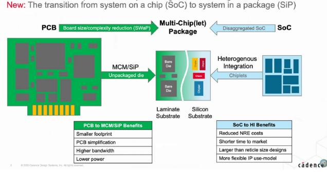
SiP/MCM vs. Chiplet-Based (Heterogeneous Integration) Architectures
