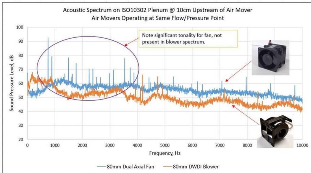
**NOTE:** The DWDI blower was not optimized for the system it was tested in. An optimized DWDI blower could have even better acoustics.
