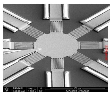
8-element PD array using interdigitated p-i-n structure
