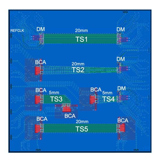
5 Test Structures 10 dies 16 Gbps D2D data rate
