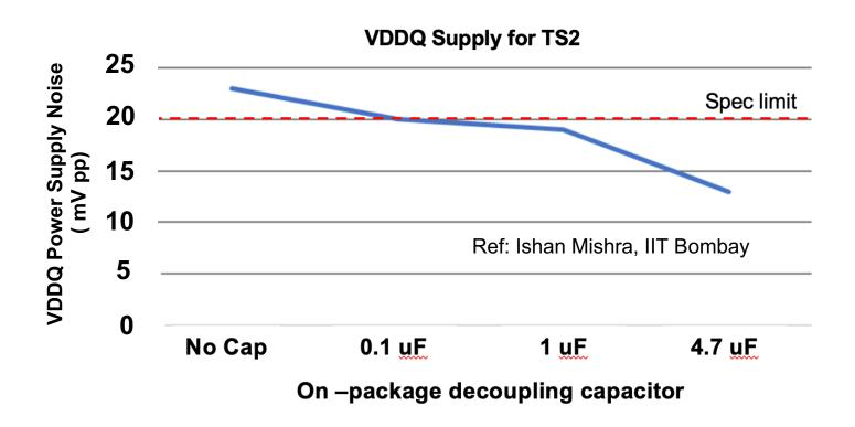
Power Integrity Specs met for all power supply rails in all test structures
