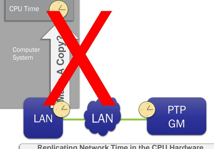
Replicating Network Time in the CPU Hardware Doesn't Scale—See next slide
