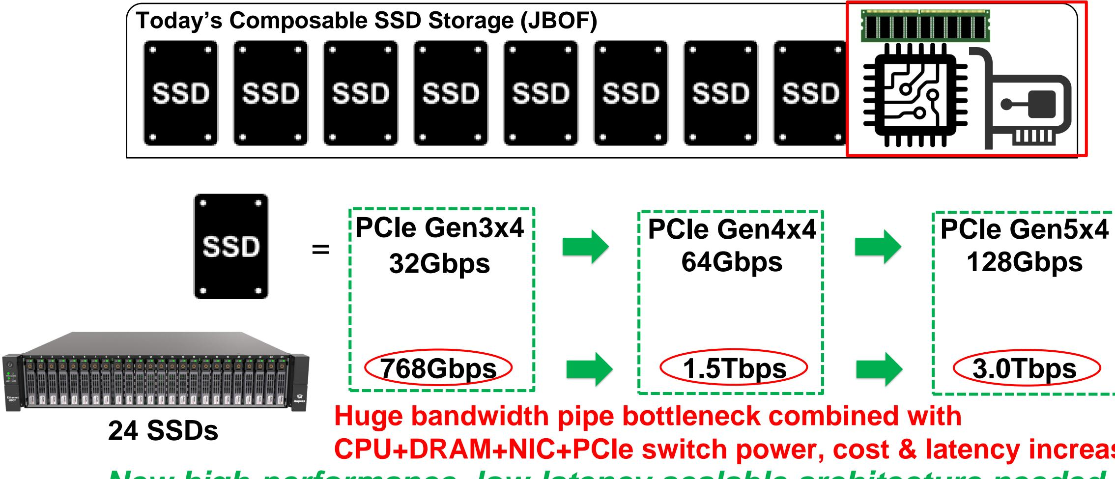
**CPU+DRAM+NIC+PCIe** switch power, cost & latency increase TCO New high-performance, low-latency scalable architecture needed
