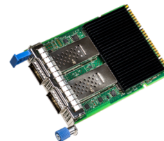
Up to 100 GbE next gen Intel® Ethernet Network Adapter for OCP NIC 3.0
