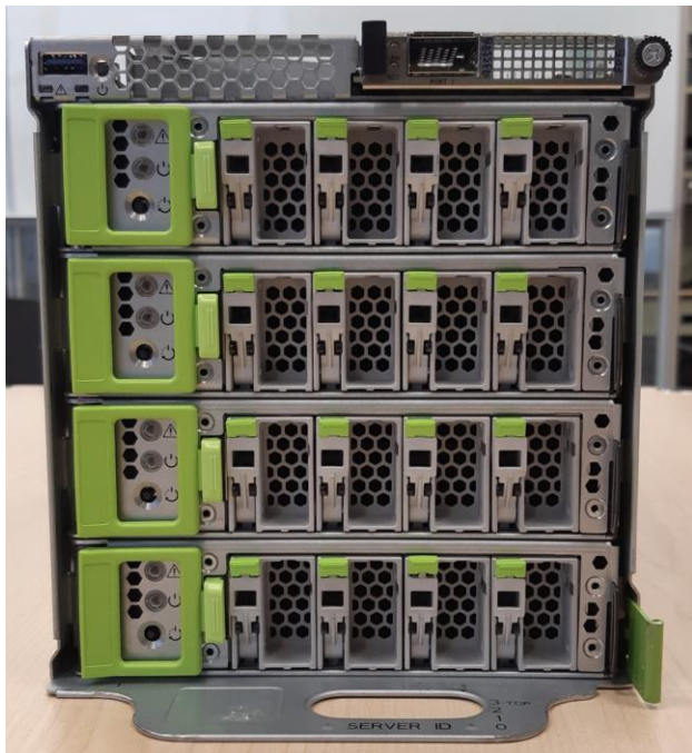
4x 10U E1.S Storage Sled Front View
