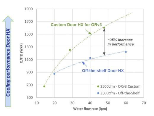
By optimizing the heat exchanger design, performance is improved.
