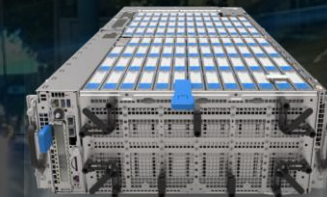
HPE CL5800 Gen9 4U 2S, 100LFF Optimized for cloud storage and big data workloads
