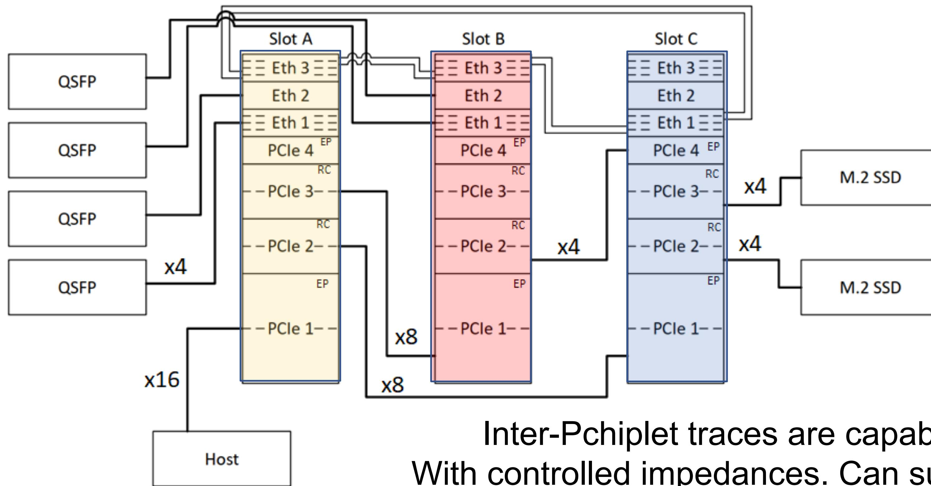
Inter-Pchiptlet traces are capable of upto 100G signaling
