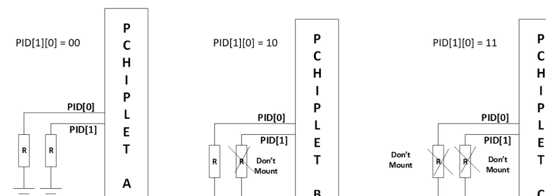
PID[0], PID[1] will be pulled up by default inside each Pchiplet
