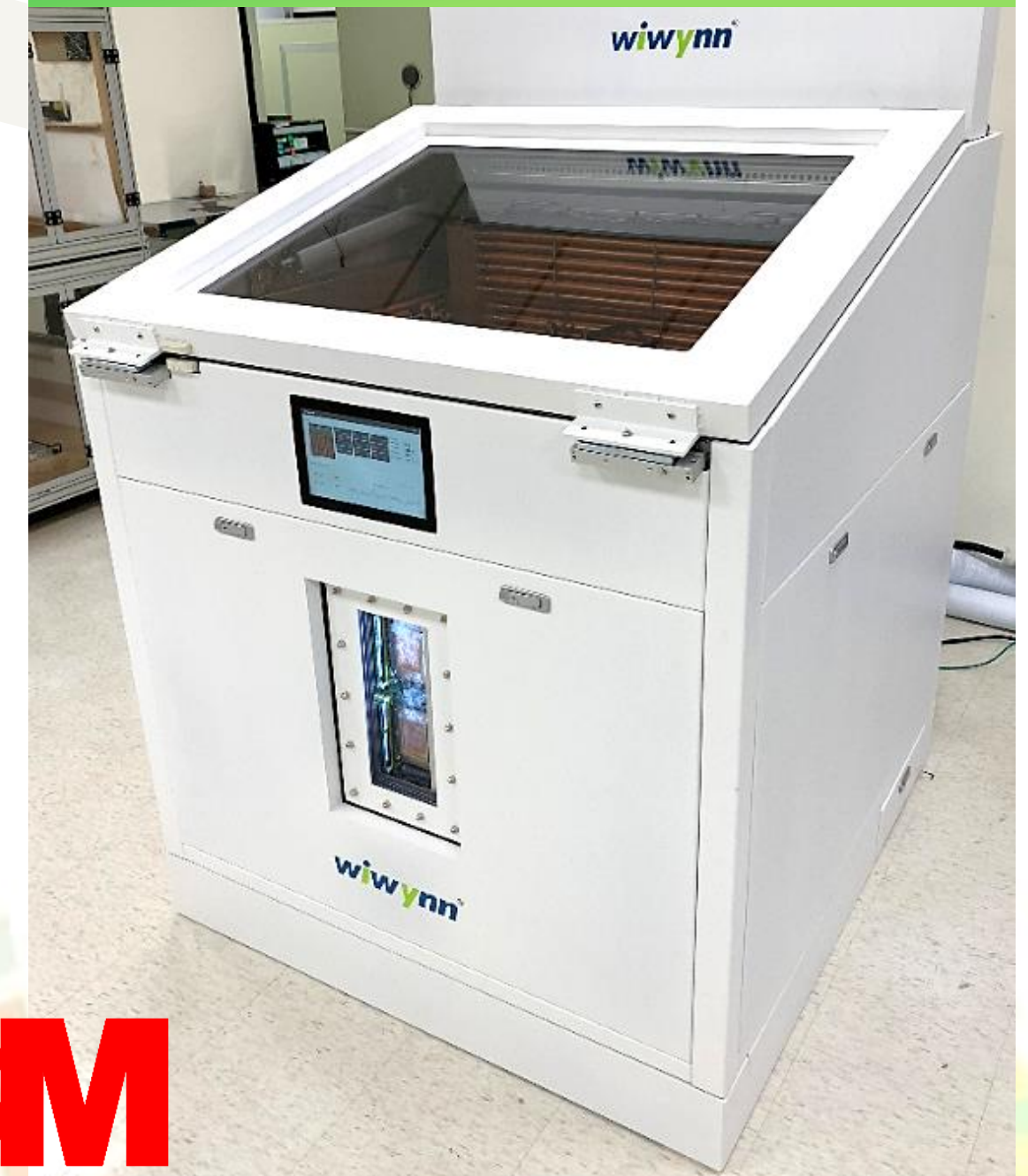
48V Immersion Cooling Solution with 3M™ Fluorinert™ Electronic Liquids
