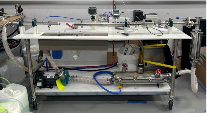
Flow impedance test fixture: tests pressure drop with different valve combinations as a function of system pressure and flow rate
