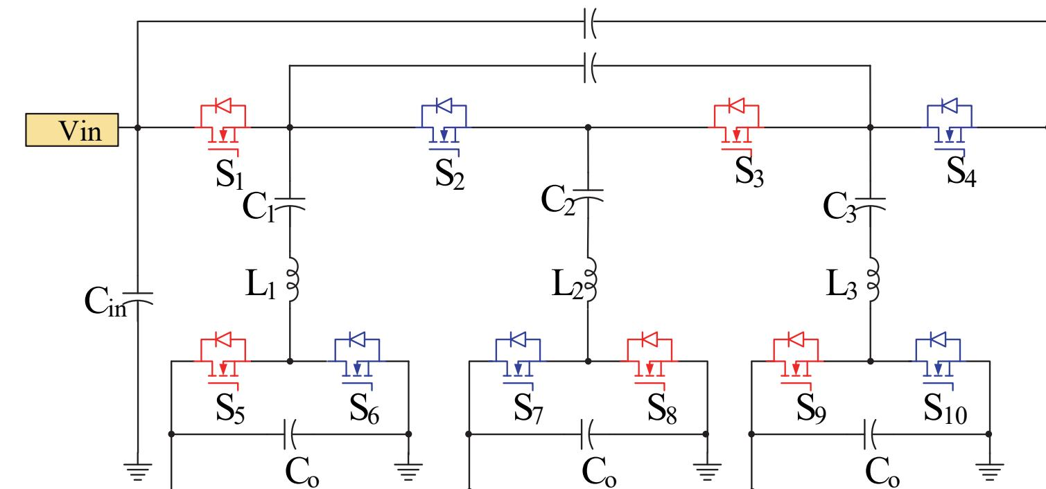
Switched-Capacitor Resonant Converter(SCRC)
