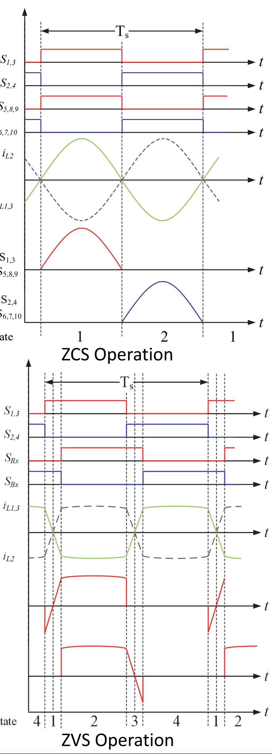
Adaptive On-time control method used to solve the unmatched resonant tank
