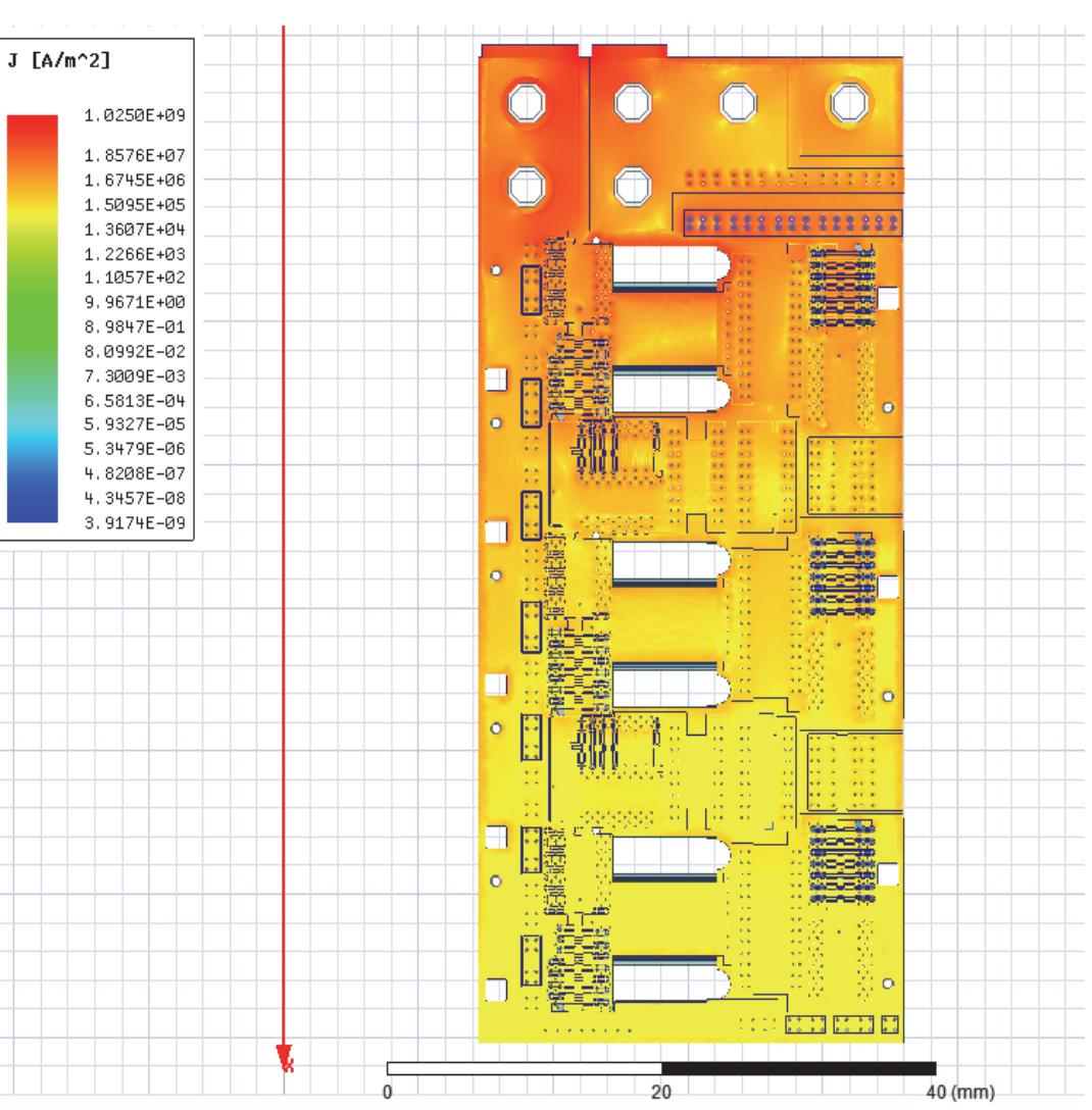
FEA software simulated PCB power loss distribution for GaN-based prototype at 450W
