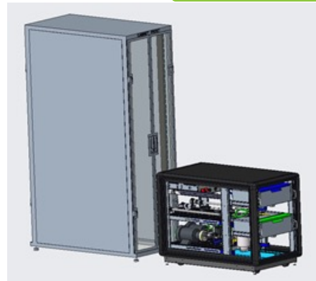
Mobile fluid-servicing cart by generic cabinet
