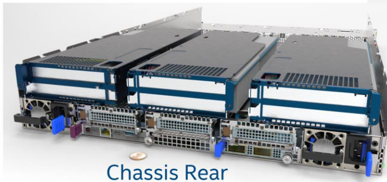
Figure 37. Typical 1U and 2U PCIe Slot Configurations for Rear Management System
