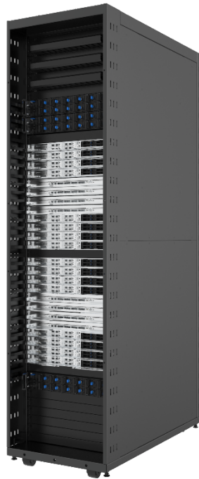
Figure 2.2 Baidu whole-rack super-node rack design example
