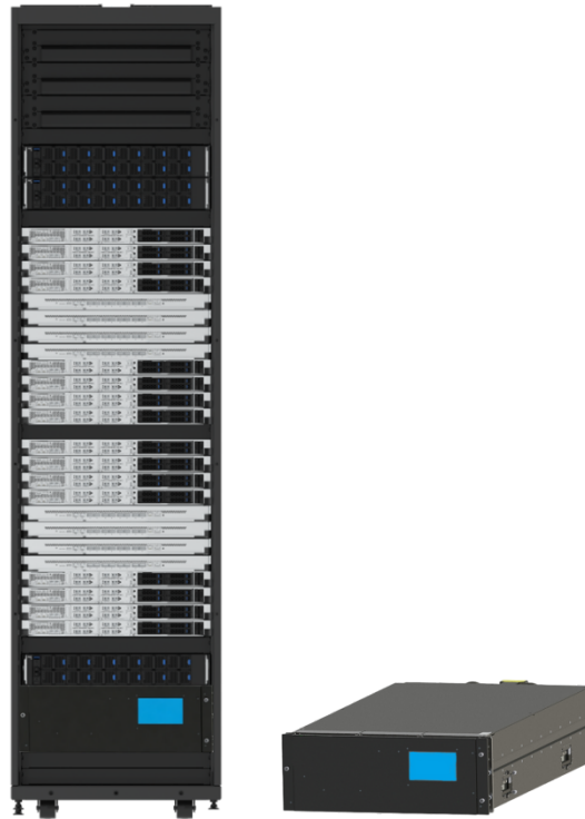
Figure 2.10 Distributed-cooling whole-rack super node
