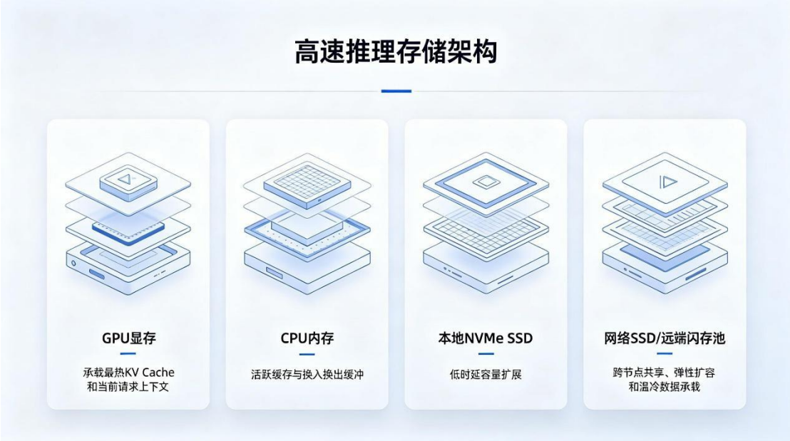
Figure 2.31 Schematic of the four-tier high-speed inference storage architecture
