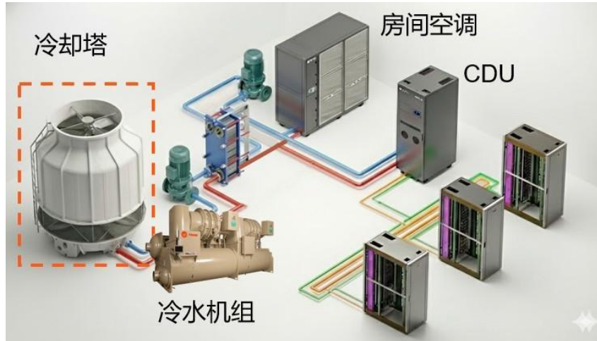
Figure 1.8 Cooling-source scheme: water-cooled chiller
