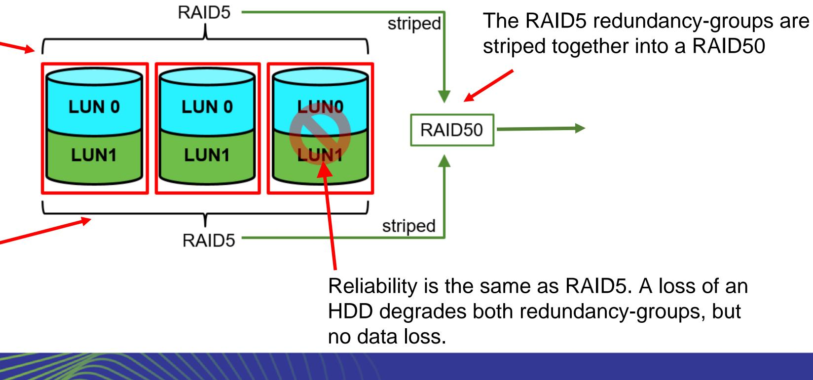
We group one LUN from each HDD into a RAID5 redundancy-group
